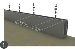
The distance between fixations is 150 mm and 50 mm from the ends, considering a chemical anchoring composed of fixing resin and a M10 threaded rod (120 mm embedded).
