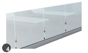
The glasses will be introduced with 10 mm space between each piece, using the foaming-adhesive seal to fill the gap inside the profile between the pieces of glass.
