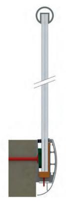
With the side-mounted solution, the profile is screwed to the slab from the outside and we add a covering profile.
