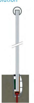
With the embedded solution, the profile is inserted by screwing it from the base with only the glass and the plastic seal remaining at sight.
