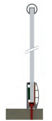
The top-mounted solution consists in screwing the profile to the ground, giving an extra protection to the glass.
