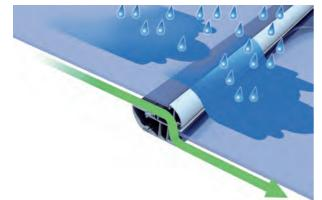
Our sliding roof is designed to be installed from the inside.
